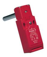
The switch includes the necessary safety-related functions, such as forced-guided contacts and a tamper-resistant mechanism, allowing machinery to be safeguarded in compliance with the machinery directive. It is sealed to IP67 and has one conduit entry, M16 or connector style.
